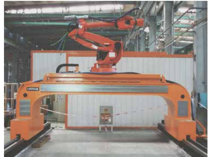
Gantry for laser robot welding with a track length of 36 m
