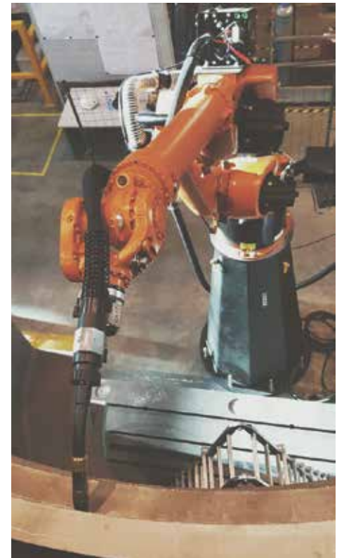
GMAW robot welding of stagnant turbine housings
