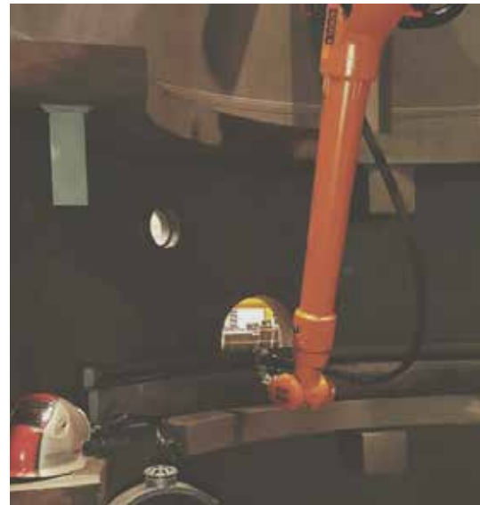
GMAW robot welding of stagnant turbine housings
