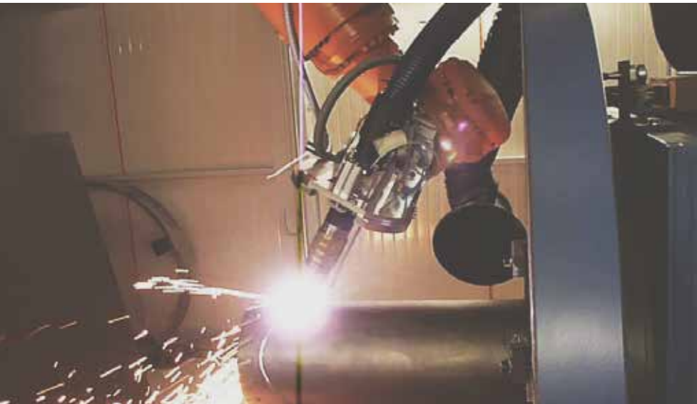
Robot plasma cutting of complex 3-D pipe contours
